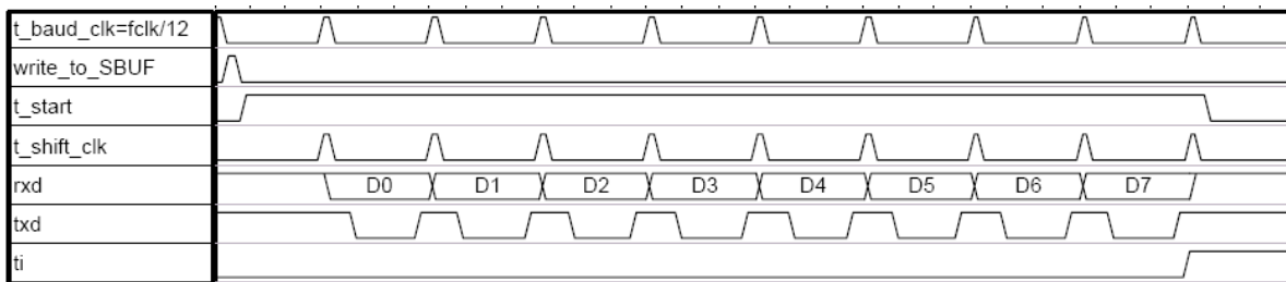
Fig. 8-1: Transmit mode 0 for Serial 0
