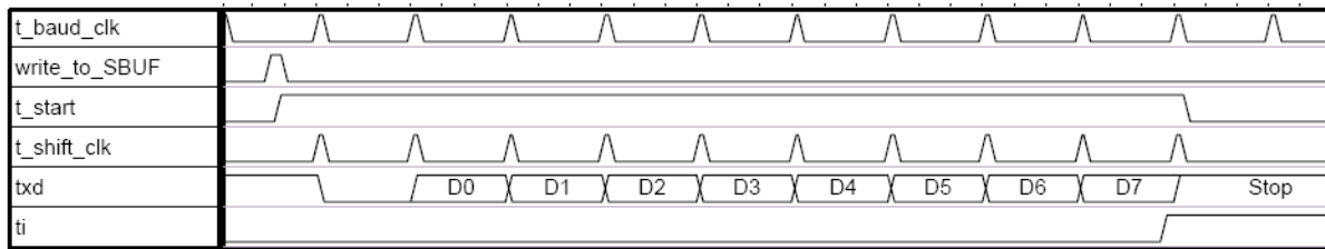
Fig. 8-3: Transmit mode 1 for Serial 0
